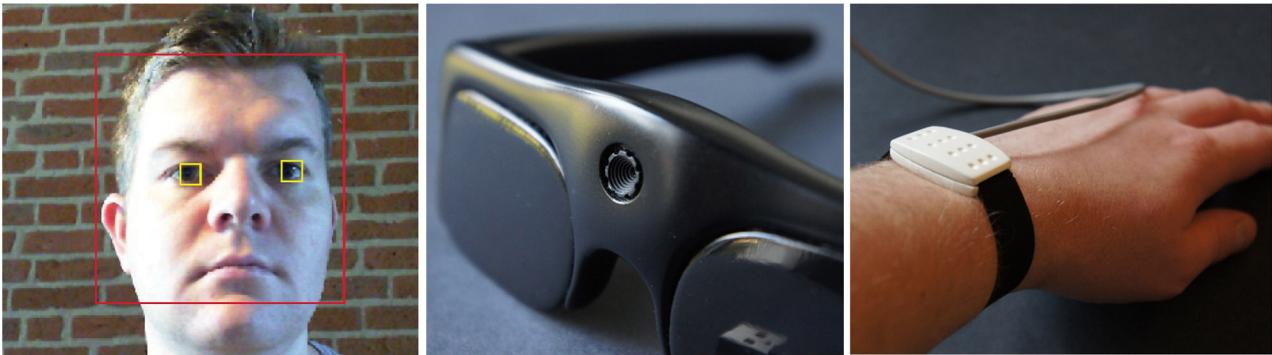
Figure 2. Three details of the Sett concept. (Left) Signal processing to detect the position of the eyes. (Middle) Integration of a camera in sunglasses to capture the image and to detect line of sight. (Right) Haptic feedback bracelet.
