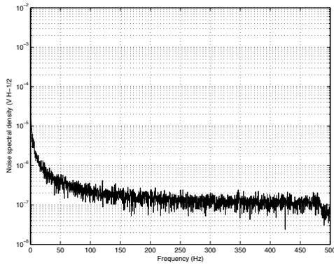
Fig. 3. Noise spectrum from the contactless sensors
