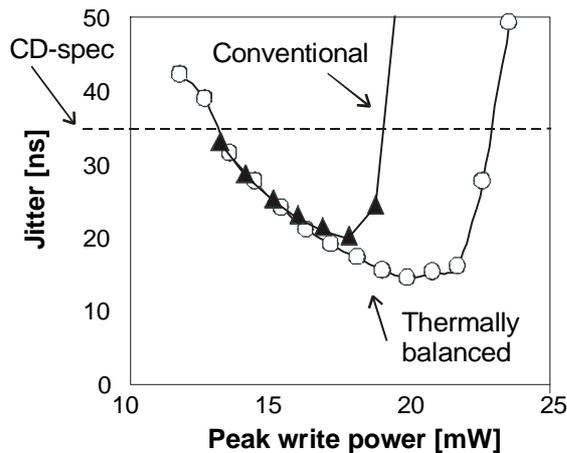
Figure 4 : Power margins when using a thermally balanced write strategy for 8X CD-R recording
