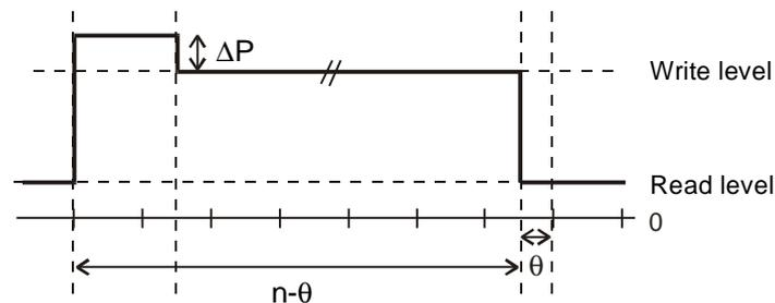
Figure 1 : Write strategy suitable for CD-recording from 1X up to 4X [1]
