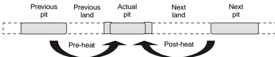
Figure 2: In-track thermal interference: the effect of pre-heat and post-heat
