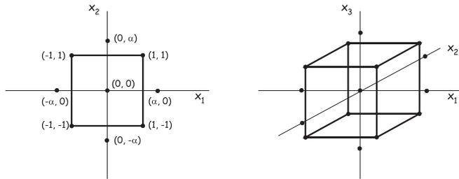
Fig. 5. Central composite designs for  $k = 2$  and  $k = 3$ .
