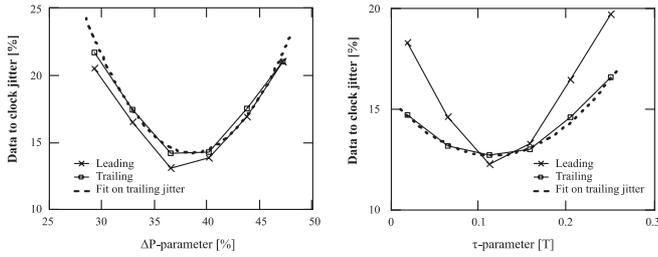
Fig. 4. Measurements on a DVD+R disc using the thermally balanced write strategy at 4×.
