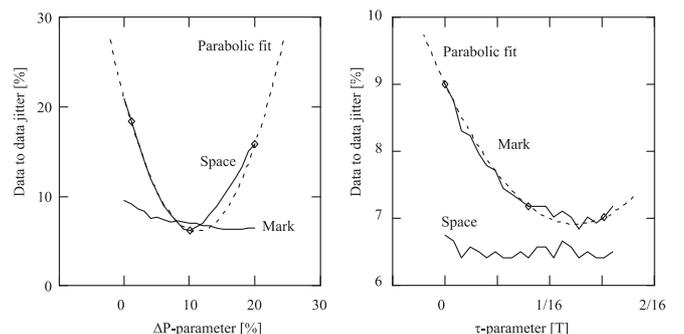
Fig. 3. Measurements on a CD-R disc using the thermally balanced write strategy at 16 $\times$ .
