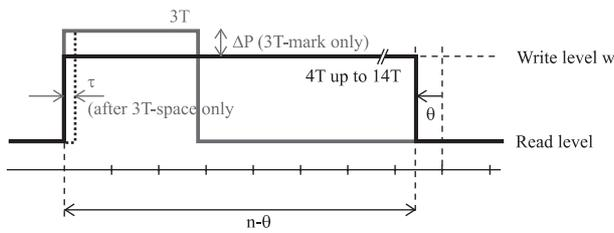
Fig. 1. Write pulse for the thermally balanced write strategy.
