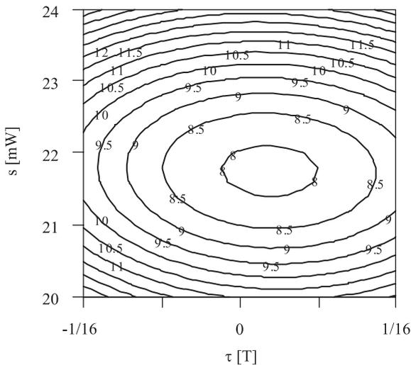
Fig. 6. Contour jitter plots for 2-factor castle strategy with a write power of 28 mW.
