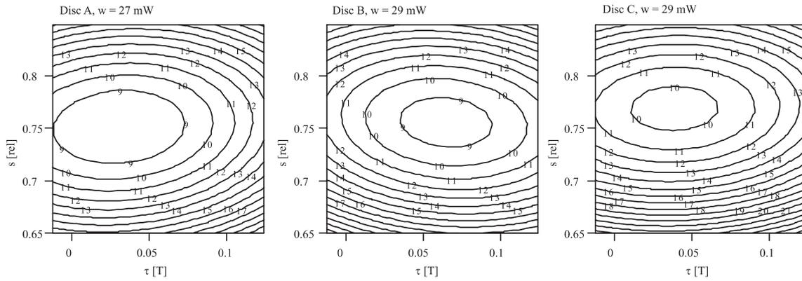
Fig. 8. Contour plots for write strategy parameters  $\tau$  and  $s$  of the castle strategy on three different discs.
