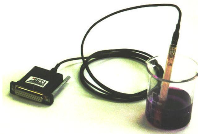
Figure 4: A complete pH measurement system
