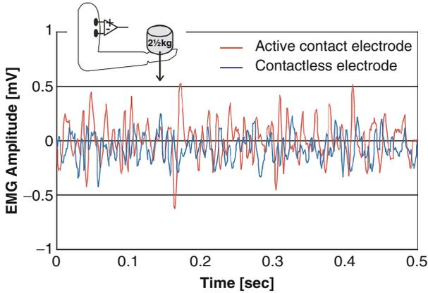
**Figure 7.** Recorded EMG signals with both an active- and contactless electrode.
