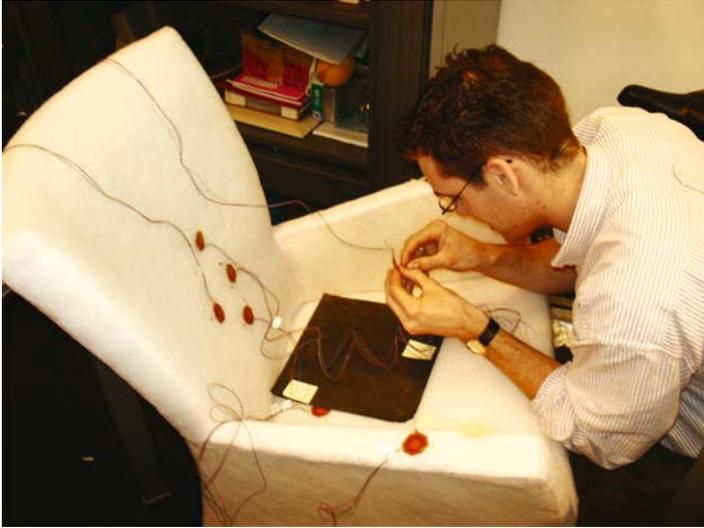
**Figure 9.** Preparing the sense chair. Amongst the sensor the capacitive groundplane is clearly visible.
