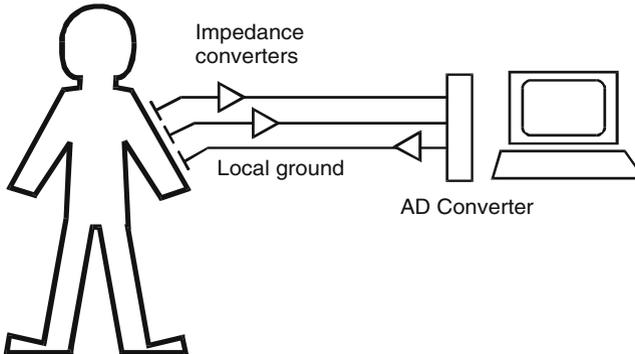
**Figure 6.** Set-up for contactless sensing of EMG signals.
