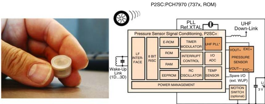
**Figure 17.** Miniature wireless temperature and pressure sensor based on NXP tire pressure sensor chip PCH7970.
