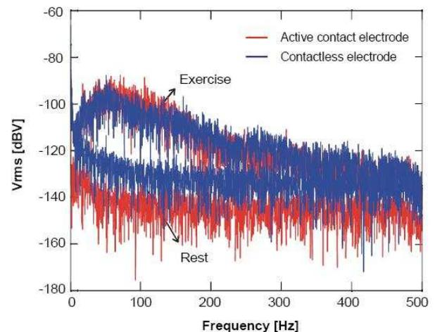
**Fig 1: spectra of the sEMG measured with both the contactless sensor and the traditional active contact sensor (Philips Research).**
