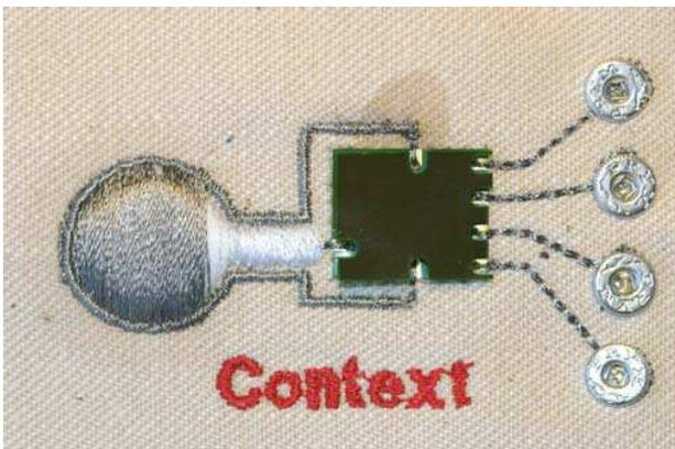
Fig 2: prototype of an embroidered sensor [15].
