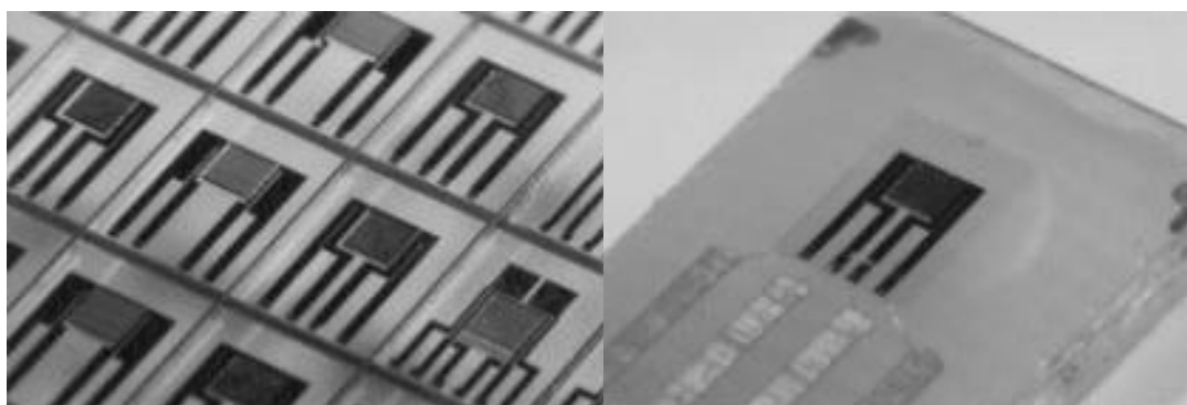
Figure 3: Photographs of realised sensor structures: just after sawing (left) and after packaging on a printed circuit board (right)
