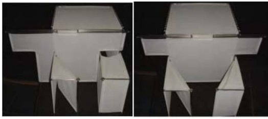
Figure 9: Model of the physical implementation of the 5-sided CAVE with the sliding doors.
