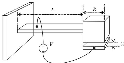
Figure 3.3-9. An electrostatically actuated mass on a spring.
