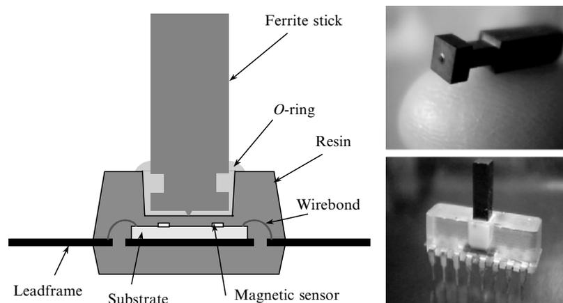
Figure 3.3-7. Integrated track pointer in DIL housing.
