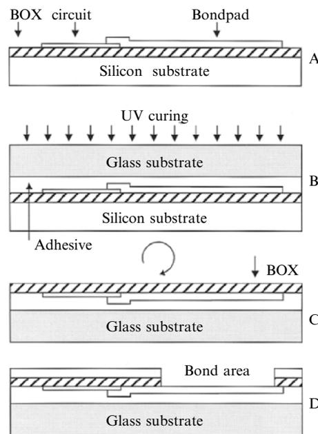
*Figure 3.3-8.* Schematic cross-section of the transfer of an SOI wafer to a glass substrate. (a) Fully processed SOI wafer. (b) Curing of adhesive by UV exposure through the glass substrate. (c) Removal of the silicon substrate selective toward the buried oxide. (d) Optional deposition of a scratch protection layer and opening of bondpads.
