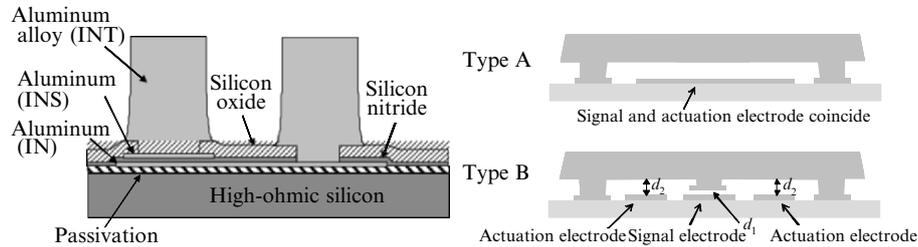
Figure 3.3-2. PASSI<sup>™</sup> cross-sectional artist impression (left-hand) and arrangements into two types of capacitive MEMS structures (right-hand).
