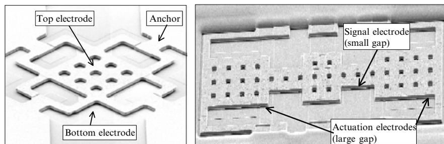
Figure 3.3-3. SEM pictures of a typical MEMS switch (left-hand) and a dual gap tuneable capacitor (right-hand).
