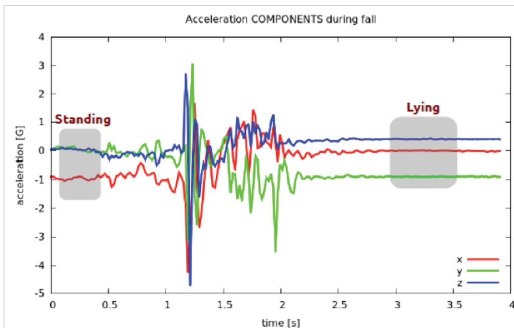
*Fig. 2.* In the project for fall detection, students made a microcontroller module that is able to detect indicators of falling for the use with elderly people
